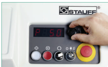
Smart programmable control panel with push/turn button and back-lit parameter display
