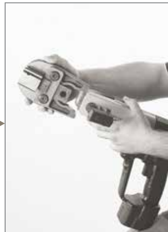
Place the jaws in the housing
