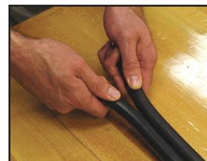
Note: It is important that the knife blade be perpendicular to the hose during this procedure so the blade cuts only the centerline of the valley (web). **EXTREME CARE MUST BE TAKEN TO AVOID CUTTING THROUGH THE COVER OF THE HOSES AND THEREBY EXPOSING THE HOSE REINFORCEMENT.** If this occurs, the hose assembly must be discarded.
