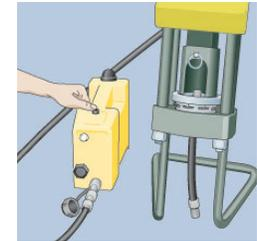
Position pusher by replacing the pin and operate pump until the die ring bottoms out. Release pressure within the pump — remove finished assembly.
