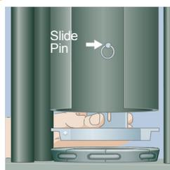
Lower the back half of the split die ring onto the dies by pulling the slide pin forward.
