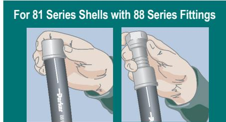
Place shell onto end of hose and make sure the end of the shell lines up with the Insertion Depth mark.
