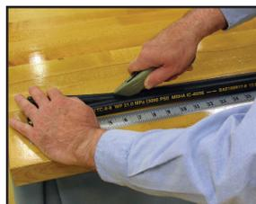
C.) Once you have a 1 to 2 inch starter cut, firmly pull each hose end apart to your required separation length.
