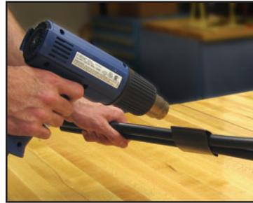
Note: EXTREME CARE MUST BE TAKEN TO AVOID EXPOSING THE HOSE ASSEMBLY TO THE DIRECT HIGH TEMPERATURES OF THE HEAT GUN WHILE INSTALLING THE HEAT SHRINK SLEEVE. LONG EXPOSURE FROM A HEAT GUN MAY ADVERSELY AFFECT THE HOSE INNER TUBE OR ITS COVER.
