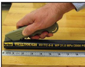
B.) To start the cut, place the blade in the center of that valley (web) drawing the knife with constant pressure.
