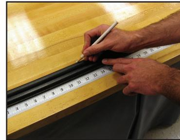
Note: If length of separation/tear back is specified from the threaded or swivel nut end of the coupling, then deduct the cut off allowance dimension for the specific style of coupling used. The cutoff allowance can be obtained from the hose fitting tables in the 4400 Catalog "B" dimension, or can be calculated by subtracting the insertion depth of the shell from the overall coupling length.
