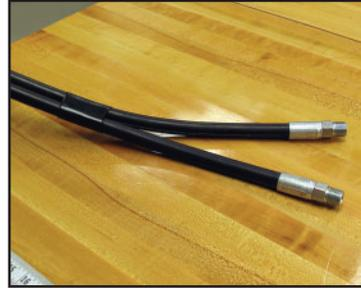
**Stopping Separation:** Parker recommends installing a heat shrink sleeve of at least 2 inches in length at the termination of the separated hose to provide protection against tearing of the valley (web) or hose covers. This heat shrink sleeve should be placed on the hose assembly prior to the crimping of the hose fittings. Once you have your heat shrink sleeve in place, use a heat gun to shrink the sleeve in place.
