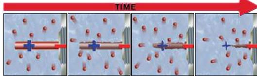
When a single potential (DC Voltage) is applied to a probe submerged in conductive liquid, metal from that probe will be lost over time via electrolysis.
