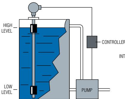
Pump-Up/Pump-Down with Intermediate Level Indication
