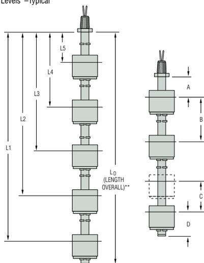
\* Actuation level distances and L<sub>0</sub> (overall unit length) are measured from inner surfaces of mounting plug or flange.
