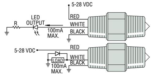
Note: Inductive loads must be diode suppressed.
