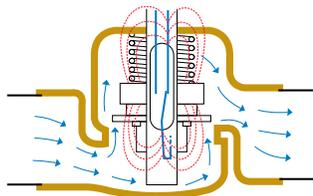
This reed switch, when actuated, can be used to operate remote alarms or indicators, or may be integrated into automatic system controls.
