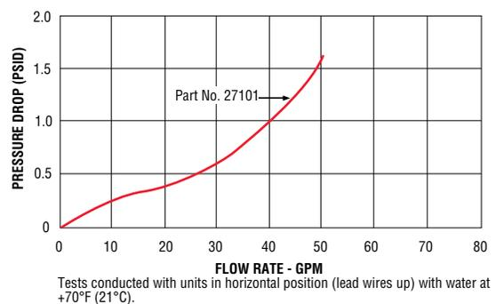
Tests conducted with units in horizontal position (lead wires up) with water at +70°F (21°C).
