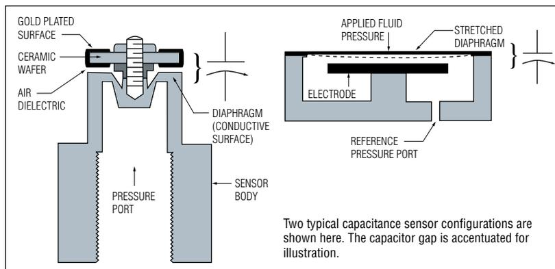
The inherent simplicity and ruggedness of this physical configuration, the fact that all wettable parts are of stainless steel or low-hysteresis ceramic, and a careful marriage of the mechanical assembly to the electronic circuitry, all combine to create a transducer that exhibits uniformly superior performance.
