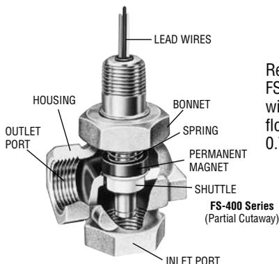
Replace an ordinary 90° pipe joint with an FS-400 Series switch to monitor liquid flow with 1% repeatability. A choice of seven flow rate actuation settings ranging from 0.75 GPM to 10.0 GPM are offered.
