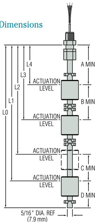
Switch actuation levels are determined following the guidelines below.
