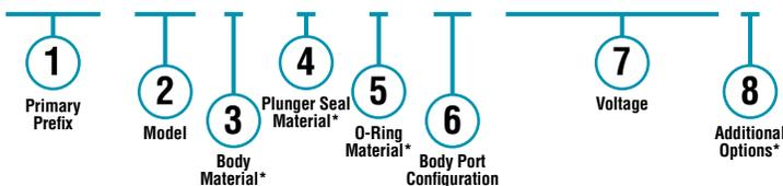
\* Blank entry indicates a "Standard" selection (430F Stainless Steel, Rulon® and Variseal®, in this case).
