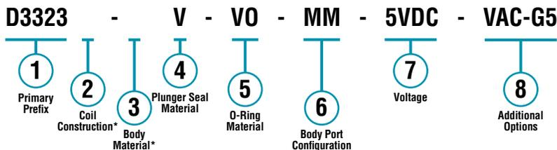
\* Blank entry indicates a "Standard" selection (Tape-wrapped, Class-B, with 18" (46cm) lead-wires and 303 Stainless Steel, in this case).
