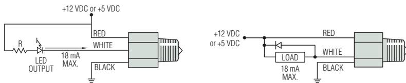
Note: Inductive loads must be diode suppressed.
