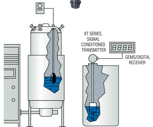
GEMS Transmitters monitor water, diesel or lube oils, chemicals and petrochemicals in industries such as pharmaceuticals, municipalities, breweries, textiles, automotive, pulp and paper and others.
