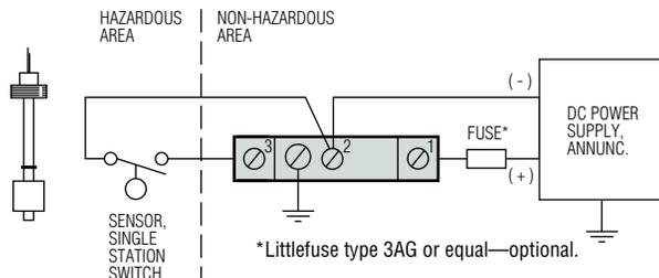
With GEMS level switch or any other non-voltage-producing device located in a hazardous area.
