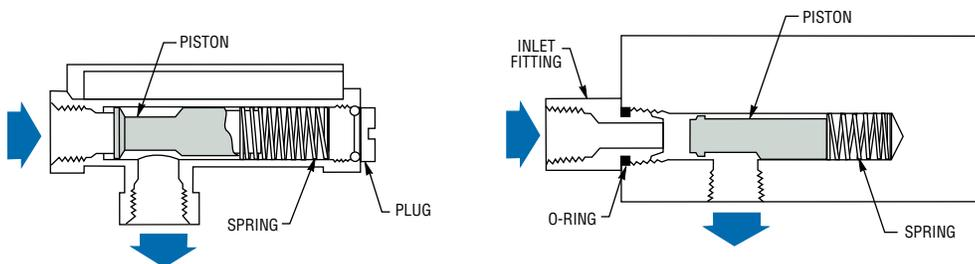
Accumulation of foreign debris should periodically be removed from these switches. GEMS' designs provide for easy piston and spring removal for this occasional cleaning. Recommended cleaning procedures are provided in the Instruction Bulletin shipped with each unit. 150 micron filtration is recommended for the FS-150 Series; 100 micron for FS-380, 50 micron filtration is recommended for all other piston type switches.
