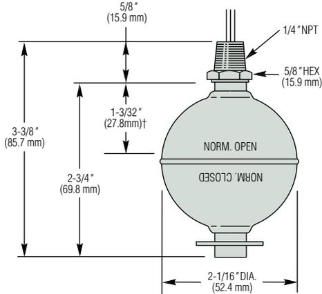
†L<sub>1</sub> = Switch actuation level, nominal (based on a liquid specific gravity of 1.0 and N.O. dry circuit – dimension will vary for N.C. circuit).
