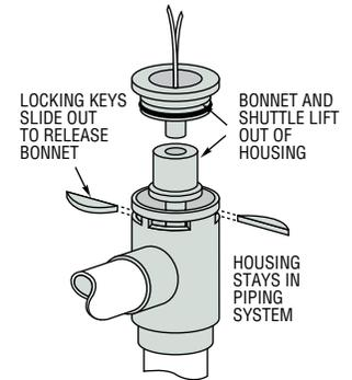
Cleanout is quick and easy. Two locking keys slide out to allow removal of a one-piece bonnet and shuttle assembly. Housing and piping are left undisturbed.
