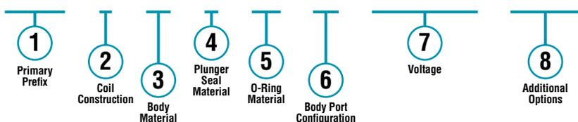
Note: After the Primary Prefix, any "-Code" may be blank when standard (blank) selections are specified.
