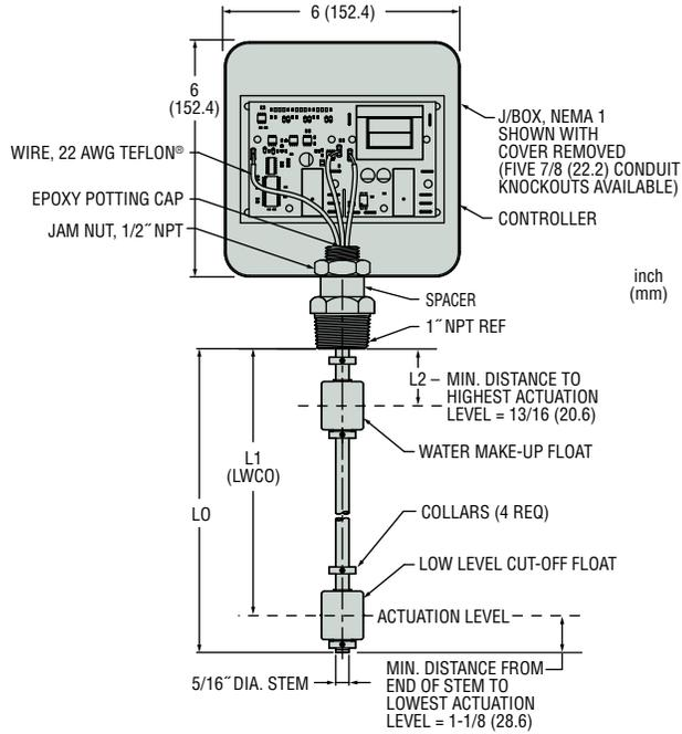
**Note:** Actuation levels are calibrated on ascending fluid levels.
