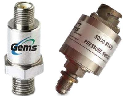
Utilizing our proven pressure sensor and ASIC design, Gems solid state pressure switches offer greater accuracy and repeatability in high shock and vibration environments. They also provide an advantage over electromechanical switches when actuations exceed 50 cycles/minute and a broad frequency response is needed. Available with a large selection of pressure port and electrical connection options.
