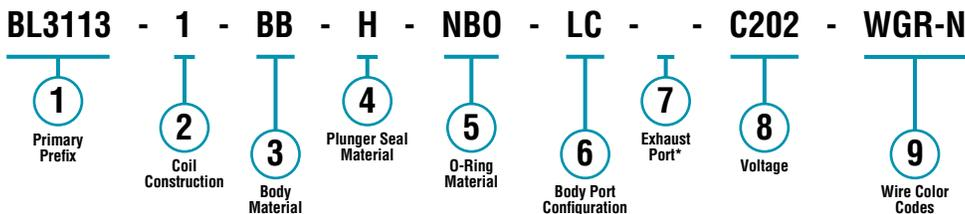
\* Blank entry indicates a "Standard" selection (#10-32 female thread, in this case).
