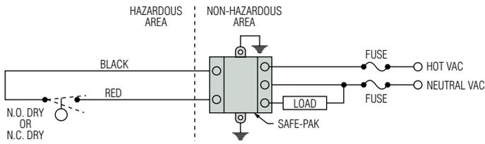
SAFE-PAK, Part Numbers 25872, 25873, 64101 or 144600 with sensor switch in hazardous location.
