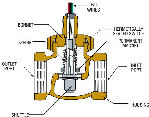
As liquid flow increases to the actuation setting, a magnet-equipped shuttle is displaced. When displaced by fluid flow, this shuttle actuates a hermetically sealed, SPDT or SPST reed switch within the unit stem. A compression spring or gravity provides shuttle return when flow decreases.
