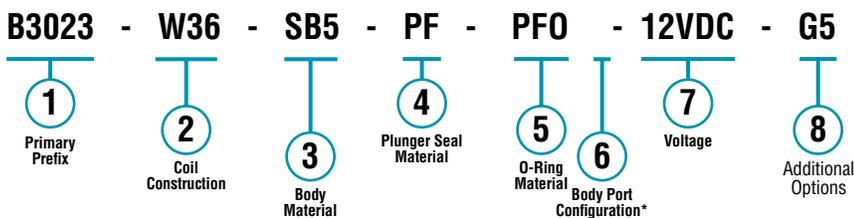
\* Blank entry indicates a "Standard" selection (1/8-27 NPT female thread, in this case).
