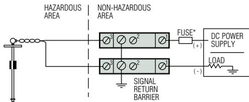
For floating leads: 65800 Series supply and return barriers for signal conditioners.
