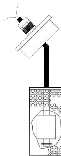
Designed to monitor hydrocarbon vapors in wells or sumps by absorbing the vapors and triggering a switch. Should not be used where vapors are continuously present. Fits in standard 2' pipe with cover.
