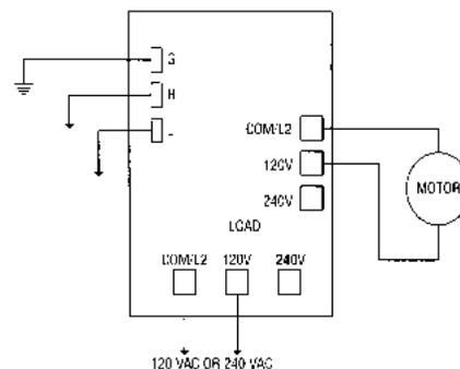
**Caution:** 19MR contacts are powered contacts. When power is applied to the 19MR controller, power may be present on relay output connections. Output voltage will be same as input voltage.
