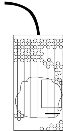
Utilizes conductivity probes and a reed switch based float switch to detect the presence of liquid and differentiate between hydrocarbons and water. When combined with Warrick DMS or TA two-channel alarm panel, the DSP-2 can discriminate between water and hydrocarbon liquids causing fault condition.
