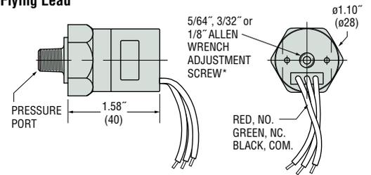
\* Adjustment screw is located under protective screw.
