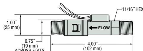
Acetal Adapters for 1/4" Quick Disconnect Male Tube Fitting Units (180°F max.)
