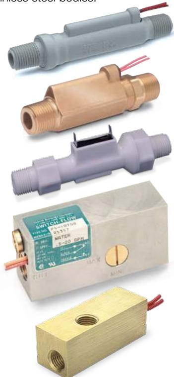
**TurboFlow®:** Ultra-compact TurboFlow® low flow rate sensors provide continual measurement ranging from 0.1 to 8 GPM (0.5 to 30 lpm). Their Hall-effect sensor delivers accuracy to  $\pm 3\%$  of reading and 0.5 % repeatability. Lightweight, they mount in any position.
