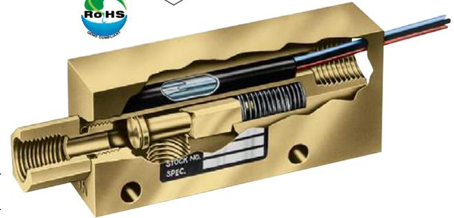
Both the FS-925 and FS-926 use a spring-loaded piston to detect positive flow with great precision. They act upon direct fluid flow and will not show "false-positive" flow indication as can happen with sensors using indirect sensing methods such as pressure measurement. The FS-926 incorporates an additional lap-fitted piston for very low flows; see below.
