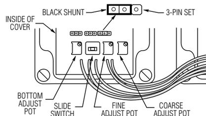
**To position decimal point:** Place black shunt over left two pins of proper 3-pin set for desired decimal in display. For no decimal, place shunt over right two pins of any set.
