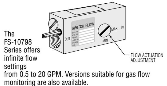
The FS-10798 Series offers infinite flow settings from 0.5 to 20 GPM. Versions suitable for gas flow monitoring are also available.
