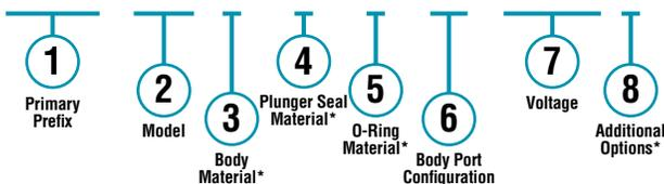
\* Blank entry indicates a "Standard" selection (303 Stainless Steel, Rulon® and Variseal®, in this case).
