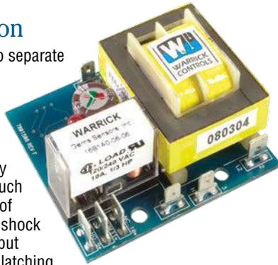
**Intrinsically Safe Controls** are solid state controls which limit current and voltage to a level incapable of igniting flammable gasses, vapors or dust. They can be used as conductivity liquid level controls or with dry contact devices such as Gems Flow and Level Switches or other non voltage storing or producing devices.
