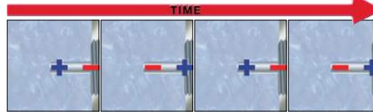
Gems applies extra circuitry to produce an alternating potential (alternating +/- DC square wave). Metal lost in one state is retrieved in the alternating state, resulting in virtually zero probe material loss.
