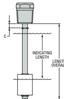
C: Minimum distance from bottom of mounting to upper float stop.
