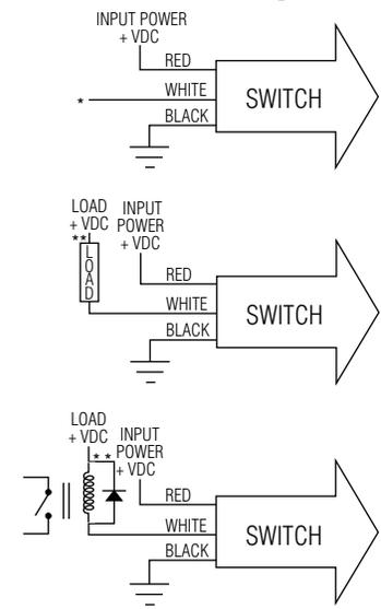
\* TTL/CMOS Output-For levels greater than 5 volts, a 10K pull-up resistor is required at the output.
