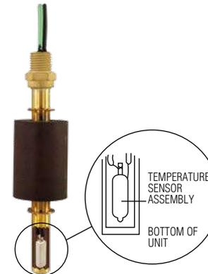
Note: End of unit stem must be submerged a minimum of 2-3/4” for level switch actuation.
