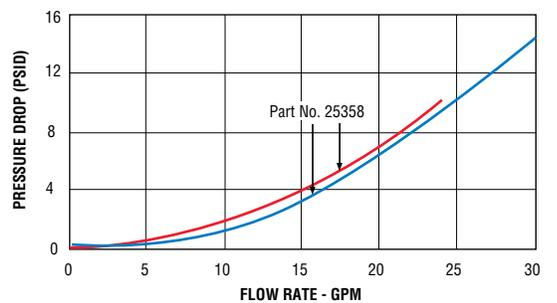
Tests conducted with units in horizontal position with water at +70°F (21°C). Data will vary slightly for vertically mounted units.
