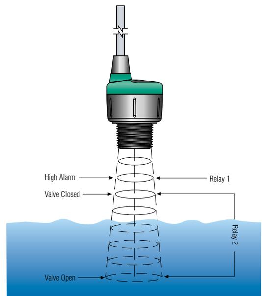
UCL-510 Series multi-point switches are designed for easy automatic tank “Hi/Lo” liquid level control. They combine non-contact continuous sensing with four SPST relays; actuation points are field adjustable in a range to 49 inches.
