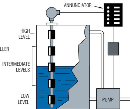
Using GEMS Custom Length level switches, junction boxes, solid-state relays and annunciators, complete liquid level control systems are easily configured.
