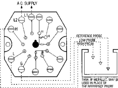
TANK, IF METALLIC, MAY BE USED IN PLACE OF THE REFERENCE PROBE
