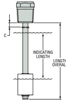
C: Minimum distance from bottom of mounting to upper float stop.
