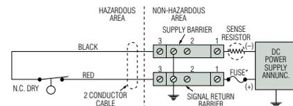
If two signal lines must be maintained above ground potential, an individual zener barrier is required per single line.
