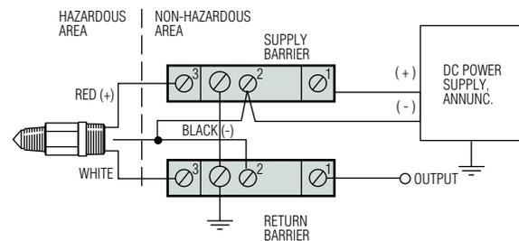
Supply and Return Zener Barriers used with GEMS EL-1100 Series electro-optical level switch.
