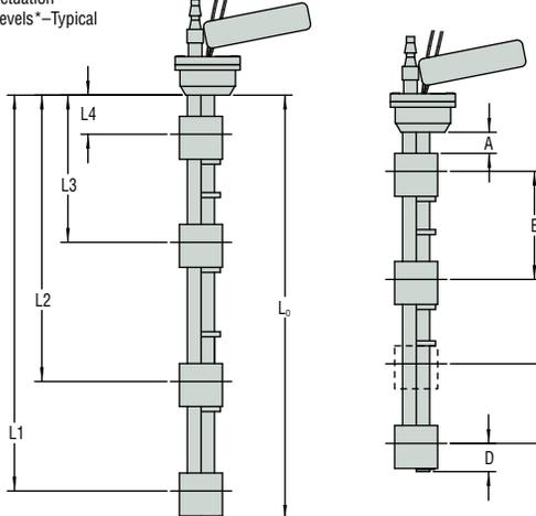
\* Actuation level distances and  $L_0$  (overall unit length) are measured from inner surfaces of mounting plug or flange. See mounting types on page B-11 for  $L_0$  reference point.
