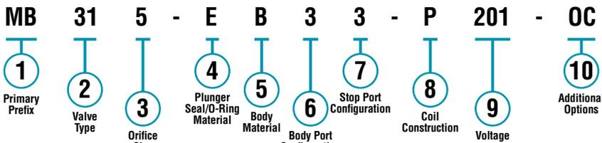
Note: After the Primary Prefix, any '-Code' may be blank when standard (blank) selections are specified.
