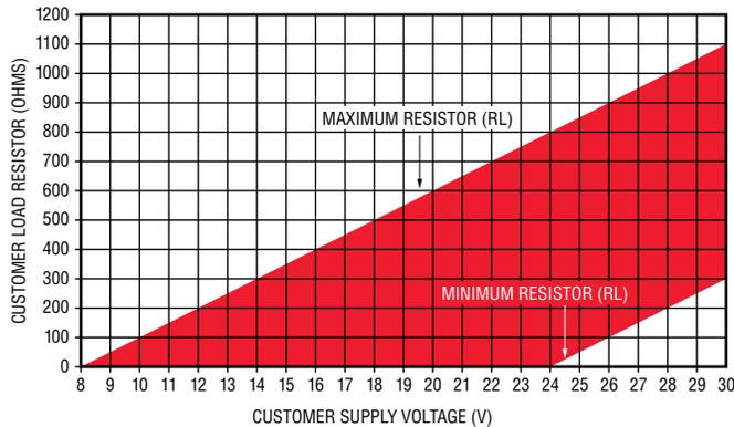
Minimum Resistor Value =  $50 \times (+V - 24)$  for  $+V > 24V$
