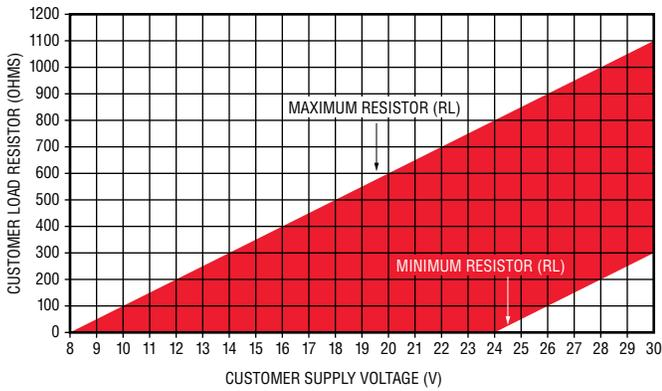
Minimum Resistor Value =  $50 \cdot (+V - 24)$  for  $+V > 24V$
