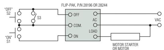
With two normally open, momentary contact push buttons (S1 and S2), the **FLIP-PAK** provides solid-state control of the motor starter or the motor itself... if load requirements are within FLIP-PAK ratings. S3 provides a safety shut-down. With S3 closed, the “ON” push button (S1) is rendered ineffective by the “OFF” override feature of the FLIP-PAK.
