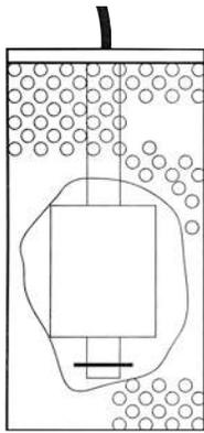
Designed to detect presence of liquid in sumps, attached access pipes, annular spaces, or locations requiring a small float-operated sensor. Two models to fit 1-1/2' and 2' standard piping.
