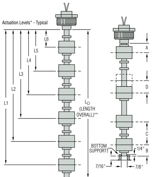
Switch actuation levels are determined following the guidelines below.
