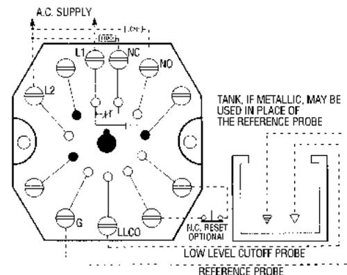
Caution: Contacts are powered. If non-powered contacts are required, request information on Series 26NM.
