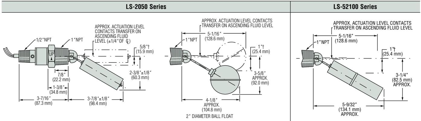
$\dagger$  Approximate de-actuation level, nominal (based on a liquid specific gravity of 1.0).
