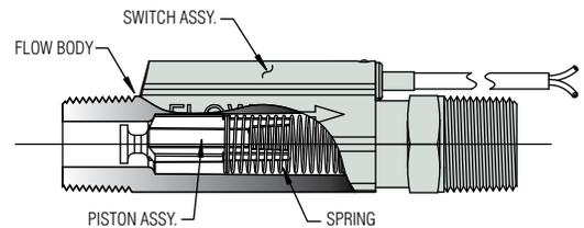
Straight design and large bore body minimizes pressure drop.
