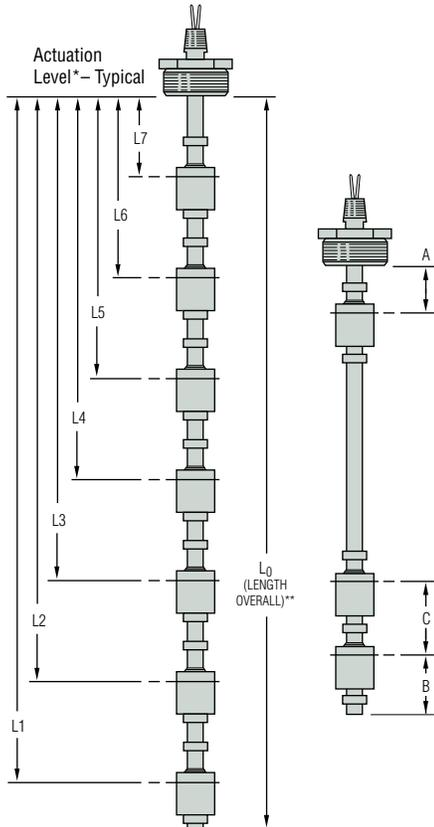
Switch actuation levels are determined following the guidelines below.
