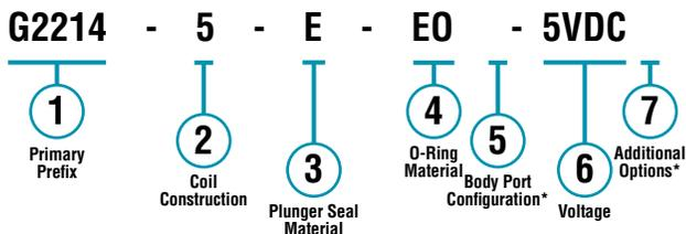
\* Blank entry indicates a "Standard" selection (#10-32 straight thread ports, in this case).
