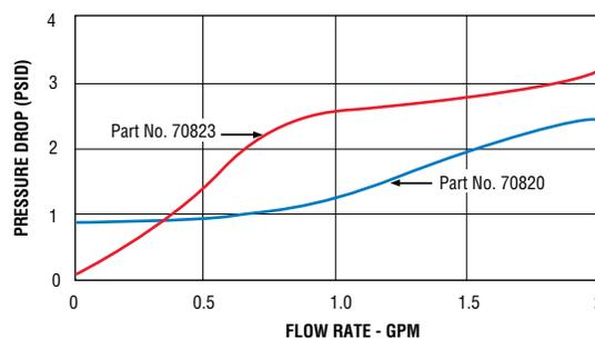
Tests conducted with units in vertical position (lead wires up) with water at +70°F (21°C).
