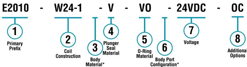
\* Blank entry indicates a "Standard" selection (#10-32 straight thread ports, in this case).
