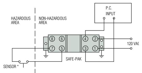
Programmable SAFE-PAK, P/N 54825, providing simple on-off functions for hazardous location, and interfacing with TTL or AC logic input of programmable controller. \*Temperature, pressure, position, flow or level.
