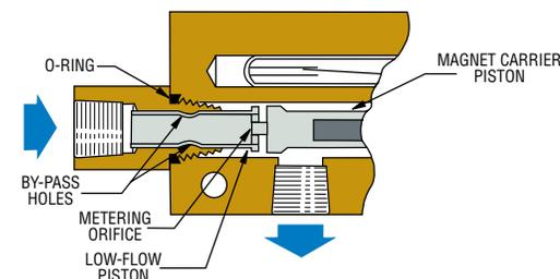
An additional, lap-fitted piston is used in Gems FS-926 Series to accurately detect low-flow rates. Calibration is determined by one or more metering holes in the end of the low-flow piston, which regulate bypass flow, and therefore the actuation setting.
