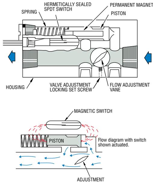
An externally rotatable vane is positioned in the main flow path within the unit. The magnet carrier piston is located in a bypass flow chamber. Pressure differential, caused by flow around the adjusting vane, displaces the spring-biased piston which actuates a hermetically sealed SPDT reed switch within the unit.
