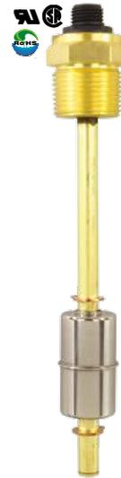
Overfill Protection for Refrigerant Tanks. The LS-700F enables safe compliance with EPA directives to recover refrigerants. These units are designed to fit standard 30# and 50# D.O.T. approved refrigerant tanks. They provide 80% full shutoff capability when used as an integral part of a recovery system.
