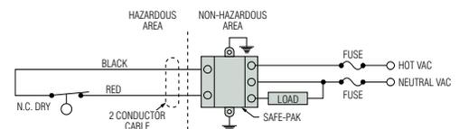
Safe-Pak® is an intrinsically safe, solid state relay
