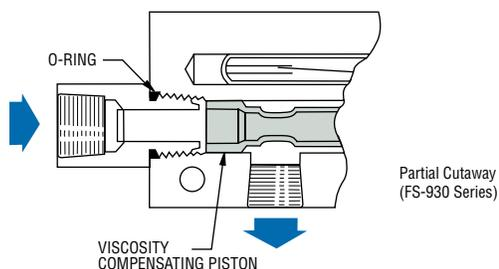
When temperatures of viscous fluids change, so do their flow properties. With viscosity lowered by increasing temperature, a greater flow is generally required to create actuation pressure differential. A unique patented piston within GEMS FS-930 Series switches accommodates these changes in fluid viscosity while maintaining accurate switch actuation. Units can detect flow rates with 20% accuracy for liquid viscosities between 40 to 1000 SSU.
