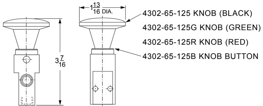
Large-diameter black plastic button is standard, for comfortable operation. Green Knob or Red Knob is available. See suffix options below. Nominal operating force is 3.75 lb. + .05 times line pressure.
