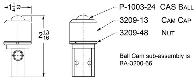
Can be operated by a cam or machine member from any angle, but pressure angle should not exceed 20° from vertical center line. Cam follower is hardened chrome alloy steel.
