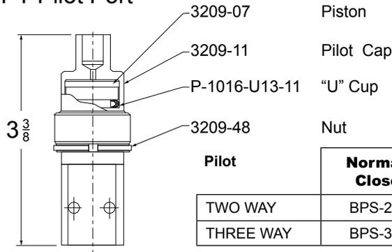
Pilot Cap Sub-Assembly is BA-3200-64
