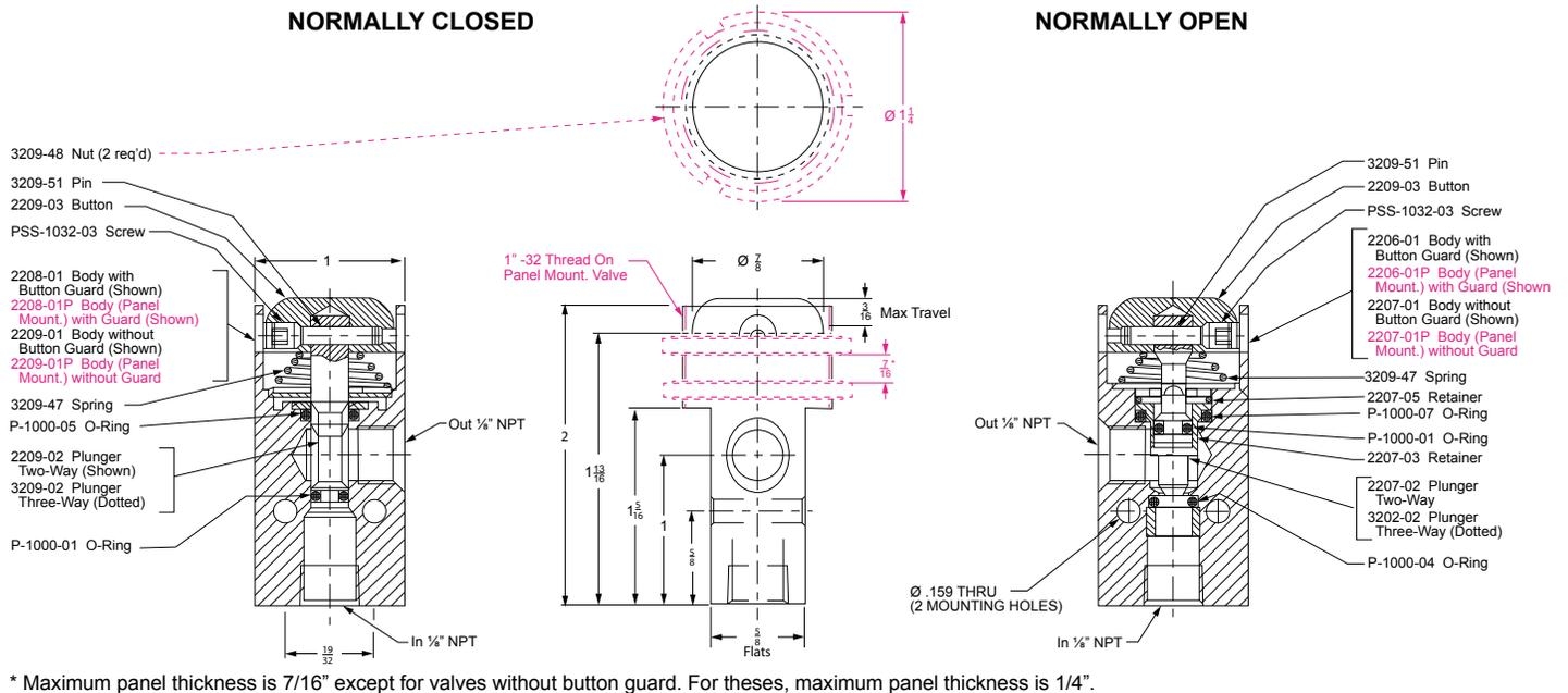
\* Maximum panel thickness is 7/16" except for valves without button guard. For these, maximum panel thickness is 1/4".
