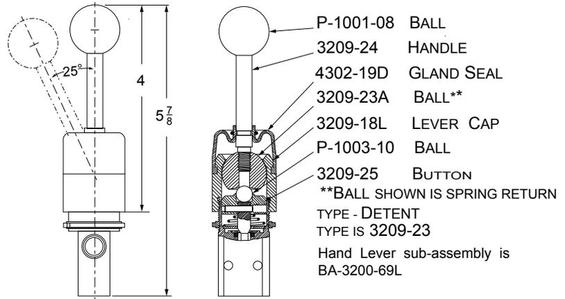
Light force, offsetting the handle 25° from vertical, is sufficient to operate
