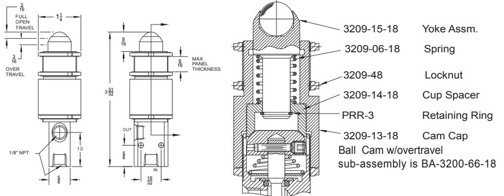
Can be operated by a cam or machine member. Has 3/16" overtravel after full actuation. This valve can be panel mounted. Pressure angle should not exceed 15° from vertical center line. Cam follower is hardened 430F stainless steel.
