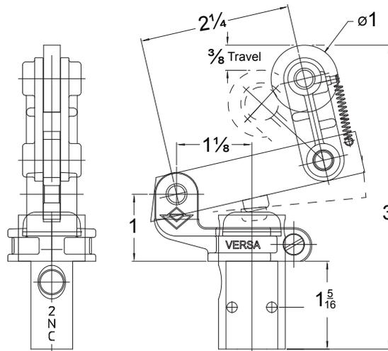
Bracket and Trip-Cam Lever is sub-assembly BA-3200-40-35.
