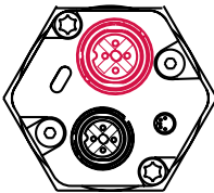
D56 Female 4-pin Bus Out
