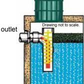
Figure 2: Diagram of installed filter and Tee Baffle. Note: drawing is not to scale.
