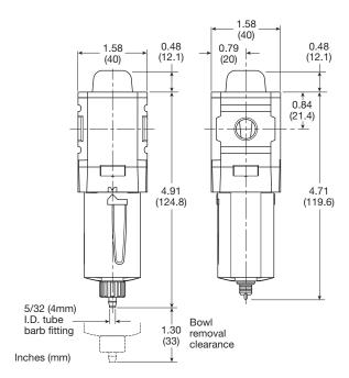
**Manual Drain Pulse Drain**
