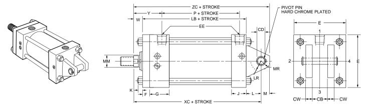
The 1", 4", 5" and 6" bore sizes have tie rod nuts at both ends as shown. Tie rods thread into cap on all other bore sizes.
