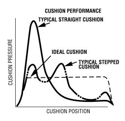
In order to cover the majority of applications. 2H/3H cylinders are supplied with profiled cushioning as standard. Final speed may be adjusted using the cushion screw. The performance of profiled cushioning is indicated on the diagram, and cushion performance for
