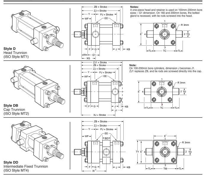
$<sup>^1\!</sup>Head$  depth increased by 5mm to accommodate port on 25mm and 32mm bore cylinders – see page 111
