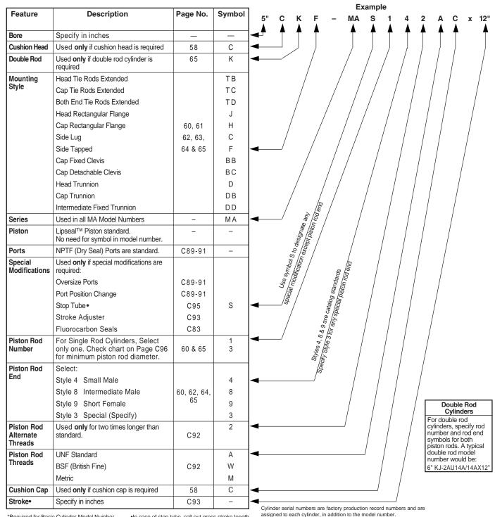
\*Required for Basic Cylinder Model Number •In case of stop tube, call out gross stroke length.
