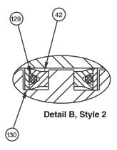
Apply "Lube-A-Cyl" to the outside diameter of the piston and seal. Then insert the piston in the cylinder body as shown in Figure 1. Next, turn the cylinder body on its side and push the piston through the barrel just far enough to expose the groove for the second seal (See Figure 2 below). Be careful not to move the
