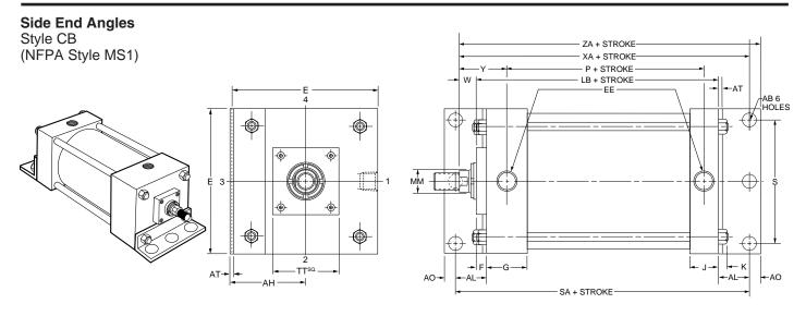
Not offered in the following sizes: 8" bore, rod codes #2, 6, 7, 8, 9 and 0; 10" bore, rod codes #8, 9 and 0.
