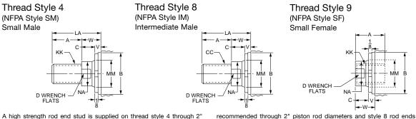
recommended through 2" piston rod diameters and style 8 rod ends are recommended on larger diameters. Use style 9 for applications where female rod end threads are required. If rod end is not specified, style 4 will be supplied.
