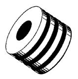
The one-piece, wide surface, nodular iron piston reduces bearing loads. The piston is piloted to ensure concentricity. Loctite is used to permanently lock the piston to the rod.
