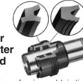
An extra-long inboard bearing surface insures lubrication from within the cylinder. Outboard of the bearing surface are two leakproof seals – The Lipseal and Wiperseal. The serrated Lipseal (primary seal) is completely self-compensating and self-relieving. It adjusts to mechanical deflections or any pressure variation from near-zero to rated operating pressure. The result is positive, no-leak sealing – regardless of conditions.
