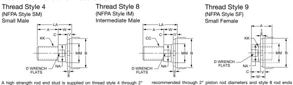
A high strength rod end stud is supplied on thread style 4 through 2" diameter rods and on thread style 8 through 19½" diameter rods. Larger sizes or special rod ends are cut threads. Style 4 rod ends are recommended where the workpiece is secured against the rod shoulder. When the workpiece is not shouldered, style 4 rod ends are
