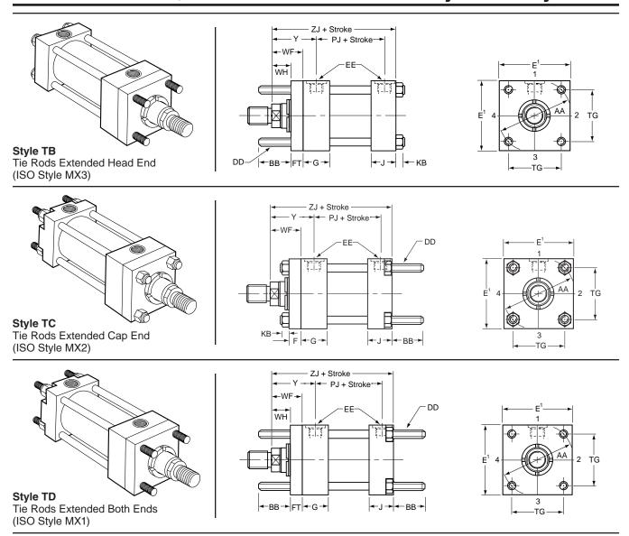
$<sup>^{1}\</sup>text{Head}$  depth increased by 5mm to accommodate port on 25mm and 32mm bore cylinders – see page 111
