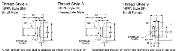
A high strength rod end stud is supplied on thread style 4 through 2" diameter rods and on thread style 8 through 13/e" diameter rods. Larger sizes or special rod ends are cut threads. Style 4 rod ends are recommended where the workpiece is secured against the rod shoulder. When the workpiece is not shouldered, style 4 rod ends are
