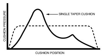
approximate the constant deceleration curve. Pressure peaks are lower than those of both the straight and tapered cushions, resulting in significantly lower hydraulic shock.
