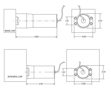
**Style F** — For LDT and LRT For 4" bore and larger only. Use Style A for 21/2" and 31/4" bore.
