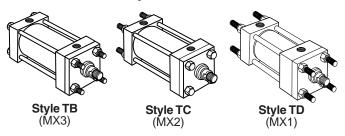
Style TB, Tie Rods Extended, is illustrated at right. Style TC, Cap Tie Rods Extended, and Style TD, Both Ends Tie Rods Extended, can be dimensioned from Style TB drawing.
