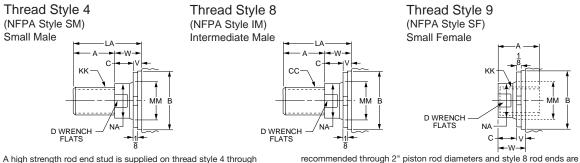
A high strength rod end stud is supplied on thread style 4 through 2" diameter rods and on thread style 8 through 19/6" diameter rods. Larger sizes or special rod ends are cut threads. Style 4 rod ends are recommended where the workpiece is secured against the rod shoulder. When the workpiece is not shouldered, style 4 rod ends are
