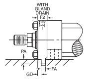
Profile of thrust key extension (with gland drain in retainer) for bore and rod combination 32mm x 22mm.
