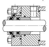
On 11/2" bore size Series 2H cyls., the drain port is located in the head adjacent to the port and on code 2 rod, the retainer thickness increases to 5/8". On 2" thru 8" bore sizes the drain port is located in the retainer as shown.
