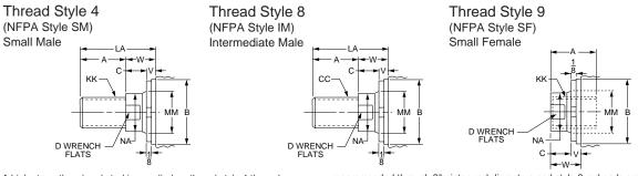
A high strength rod end stud is supplied on thread style 4 through 2" diameter rods and on thread style 8 through 13/s" diameter rods. Larger sizes or special rod ends are cut threads. Style 4 rod ends are recommended where the workpiece is secured against the rod shoulder. When the workpiece is not shouldered, style 4 rod ends are
