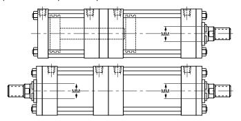
Reduced operating pressure is required for this construction. Contact factory.
