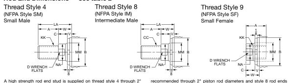
A high strength rod end stud is supplied on thread style 4 through 2" diameter rods and on thread style 8 through 13/s" diameter rods. Larger sizes or special rod ends are cut threads. Style 4 rod ends are recommended where the workpiece is secured against the rod shoulder. When the workpiece is not shouldered, style 4 rod ends are
