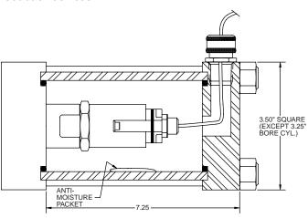
**Style D** — For LDT Basic and Intergral Cap. Specify connector type (not available on 2" bore).
