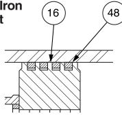
For elevated temperature service above +250°F. (+121°C) specify Class 5 seals plus a non-studded piston rod end thread and a pinned piston to rod connection. This recommendation should also be followed when ordering spare piston and rod assemblies. Class 5 seals can operate up to a maximum of +400°F. (+204°C) with reduced service life.
