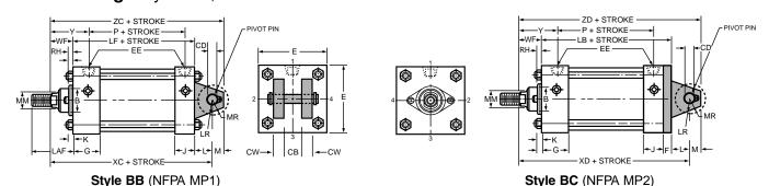
Tie Rods thread into Cap on 11/2", 2", 21/2" & 31/4" bore sizes as shown. Larger sizes have Tie Rod Nuts at both ends.
