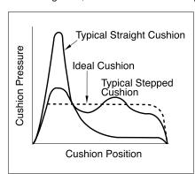
advantages. In order to cover the majority of applications, HMI cylinders are supplied with profiled cushioning as standard. Final speed may be adjusted using the cushion screws. The performance of profiled cushioning is indicated on the diagram, and cushion performance for each of the rod sizes available is illustrated
