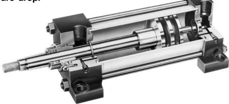
Parker engineers have developed a new concept in air cylinder cushions...the "check seal". The new Parker check seal cushion combines the sealing capabilities of a lipseal for efficient capture of air for effective cushioning with check valve action for quick stroke reversal.
