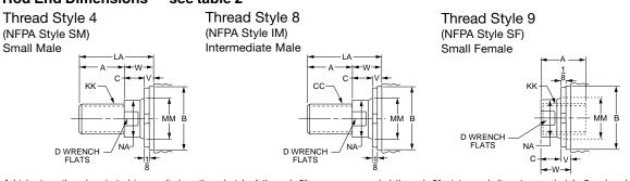
A high strength rod end stud is supplied on thread style 4 through 2" diameter rods and on thread style 8 through  $13/_6$ " diameter rods. Larger sizes or special rod ends are cut threads. Style 4 rod ends are recommended where the workpiece is secured against the rod shoulder. When the workpiece is not shouldered, style 4 rod ends are
