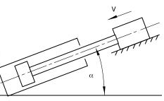
Selected bore/rod 160/70mm (No. 1 rod). Cushioning at the cap end.
