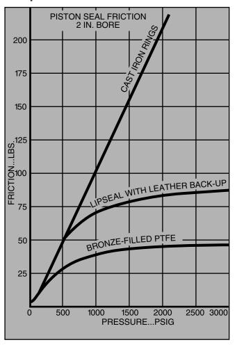
Virtually zero leakage. The HI LOAD piston assembly means virtually zero leakage with hydraulic and/or water base fluids because of the continuous bronze-filled PTFE rings with a homogenous inner ring of Nitrile rubber to apply seal preloading. The Nitrile expanders provide enough initial radial force to eliminate low pressure leakage. At higher pressure (above 2,000 psi) the seals are pressurized underneath, and are therefore dynamically self-sealing just as cast iron rings are.
