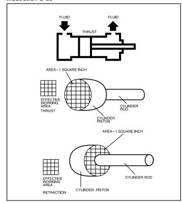
**Pistons** vary in design and materials used. Most are made of cast iron or steel. Several methods of attaching the piston to the rod are used. Cushions, are an available option on most cylinders and most often, can be added with no change in envelope dimensions.
