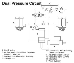
This basic circuit is for a dual pressure system supplying pressure to a double-acting work system. The circuit may be readily
