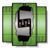
**Load-Lock Design...** is simple and effective. The drive lug configuration is tapered from top to base, as are the mating lugs of the opposing coupling hub. Under load, the insert conforms to the tapers, inter-locking the two hubs. This load-lock design protects bearings and equipment by eliminating end thrust in both directions.... and it requires only one set-screw in each hub.
