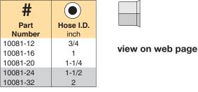
81 Series consists of a 10081 crimp shell and is completed by adding any 88 Series Fittings. See Equipment Section for complete 81 Series Assembly and Crimping instructions.
