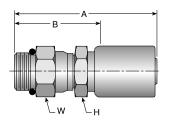
Fitting allows minor movement under pressure to relieve stress on hose but is not to be used on extensive or continuous swiveling.
