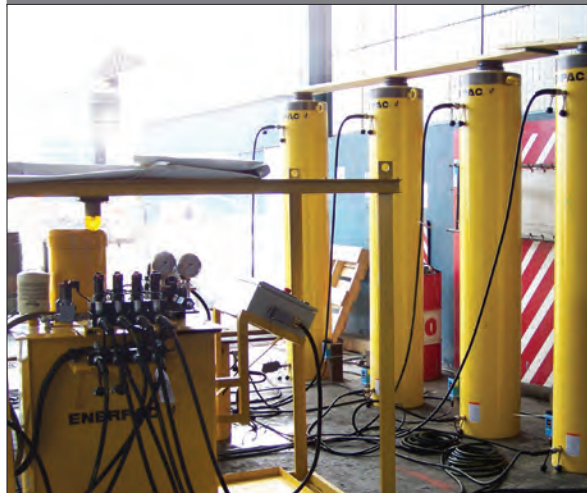
▲ Custom 500-ton cylinders with 72-inches of stroke for lifting electric rope shovels.
