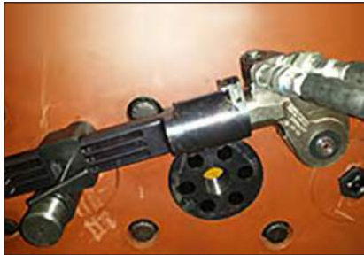
◀ Custom hydraulic torque wrench for a fracking pump.
