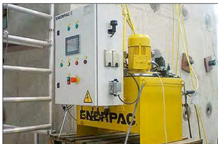
◀ Custom pumps with control packages.
